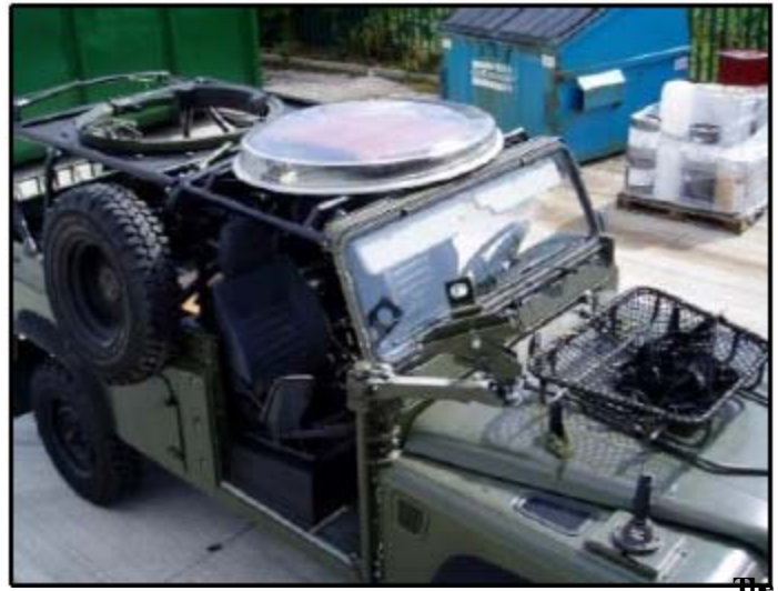
Mobile satcom terminal unit by ERA technology can be used for military applications.
