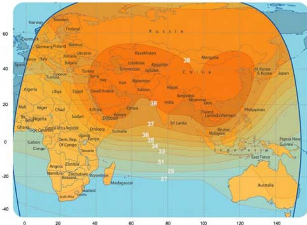
14C-Band transponders @ 36MHz polarization: linear (H & V) downlink frequency range: 3.400 GHz - 3.700 GHz uplink frequency range: 6.425 GHz - 6.725 GHz
