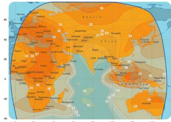
14C-Band transponders @ 36MHz polarization: linear (H & V) downlink frequency range: 3.700 GHz - 4.000 GHz uplink frequency range: 5.725 GHz - 6.025 GHz
