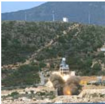
A static test firing of the Zefiro 23 second-stage engine of Europe's new Vega launch vehicle was conducted on Monday 26 June 2006, at the Italian Ministry of Defense test centre in Salto di Quirra, Sardinia. (Credits: ESA-S. CORVAJA photo)
