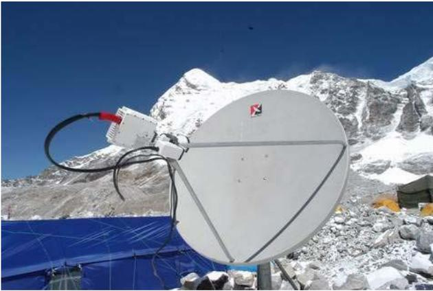
Now fast forward to today. Broadband VSAT terminals operating with 2 to 8 Mbps inbound and up to 45 Mbps outbound carriers; remotes barely larger than my laptop computer, with an integrated IP router, IP acceleration and can receive streaming video. Voice, no problem; just plug in VOIP phones or connect to a PBX. Oh yes—almost forgot—IP video-conferencing works great too.
