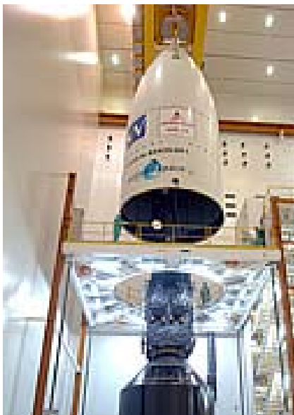
The Arian 5 payload fairing is lowered over WildBlue-1 and the SYLDA 5 dispenser Credit: Arianspace
