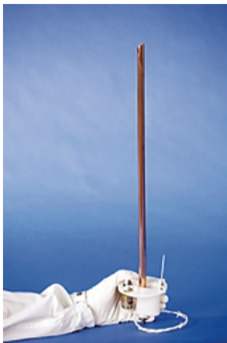
Northrop Grumman's RADARSAT Constellation Mission antenna unit in deployed state.
