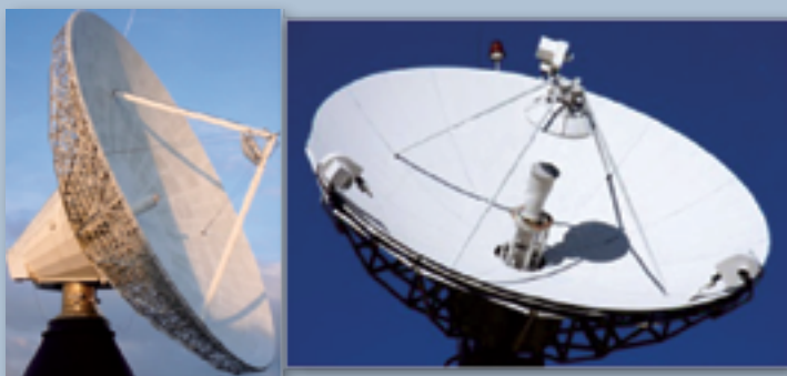
Figure 3. From left to right, Cassegrain and Gregorian antenna.
