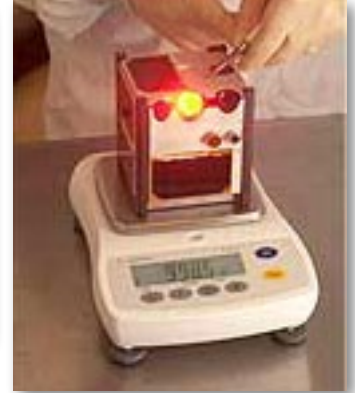
If this CubeSat weighed two more grams, it would be classified as a nanosatellite instead of a picosatellite. Photo by Eric Hamburg
