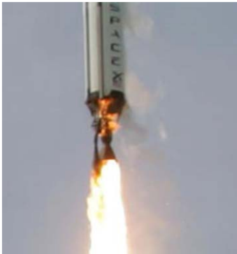
An engine close up shows the fire that doomed Falcon 1 on its maiden flight. (Thom Rogers/SpaceX photo)
