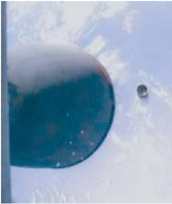
SpaceX Falcon 1's first stage falling back toward Earth with the second stage rocket engine in the foreground. (SpaceX photo)
