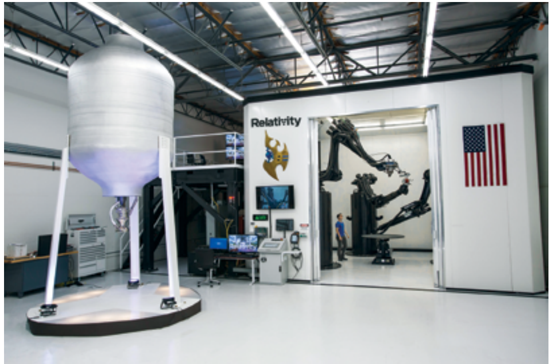
Relativity's Stargate, the largest metal 3D printer in the world — Built for rockets. Photo is courtesy of the company.
