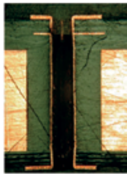
b) Coaxial via through core
