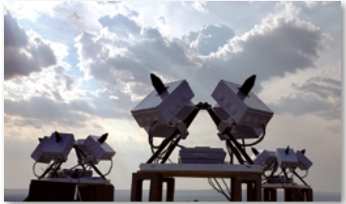
ATLAS Links, an electronically steered, lightweight and easily deployable array ideal for high volume or operationally limited environments. Links weighs only 55 pounds and can be carried in a backpack.
