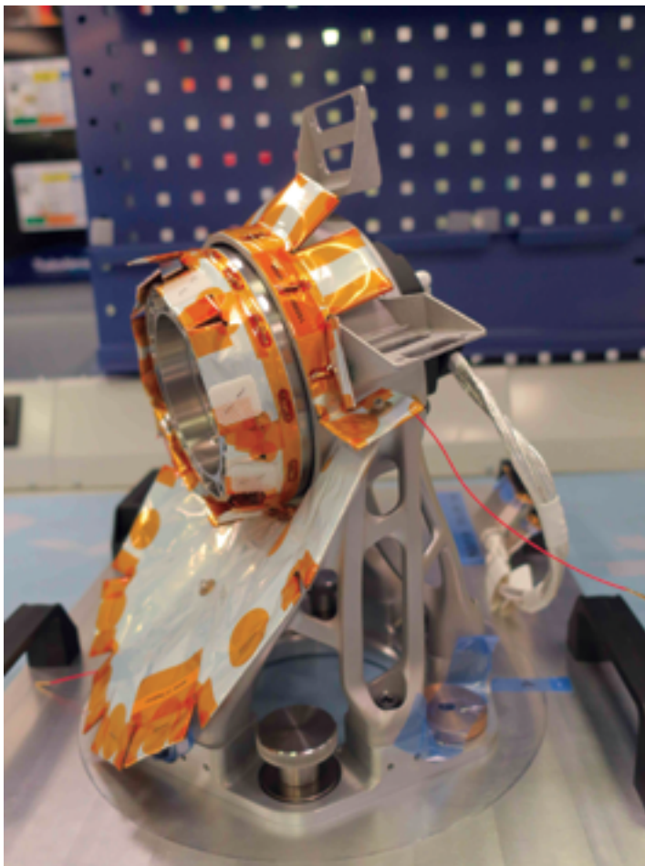
Spacebus Neo will feature four reaction wheel brackets made of aluminum and 16 antenna
