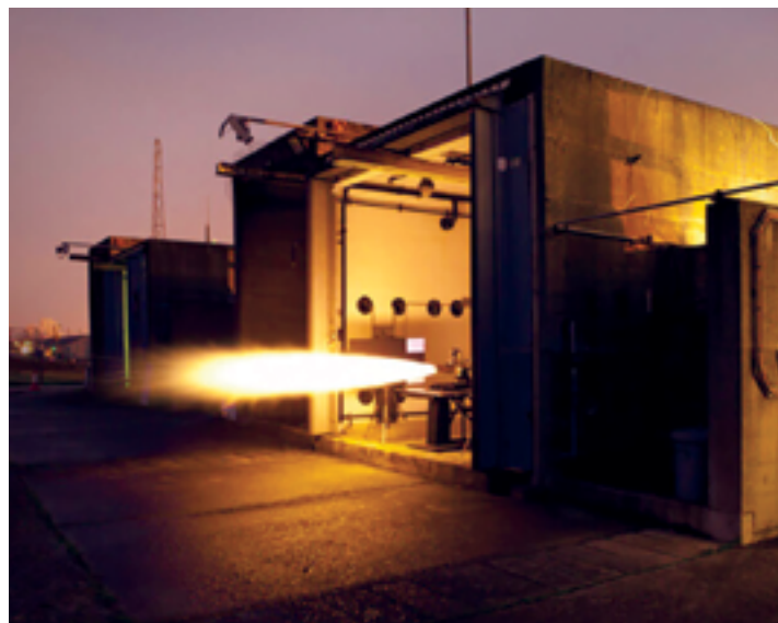
A test firing of the Sabre rocket engine. Photo is courtesy of Reaction Engines.
