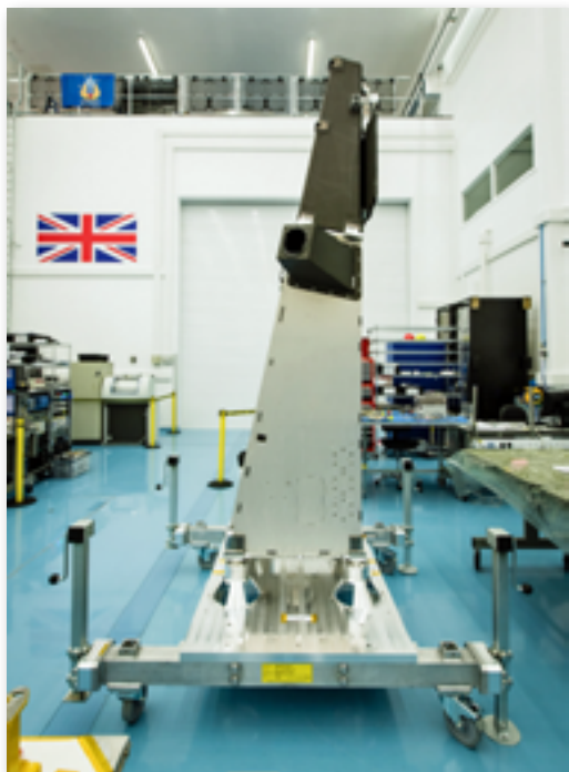
The NovaSAR-S structure in the Assembly, Integration and Test Hall. The spacecraft's structure is made from aluminium and carbon fiber panels, manufactured at the Composites Facility in Bordon. Photo is courtesy of Airbus Defence and Space.
