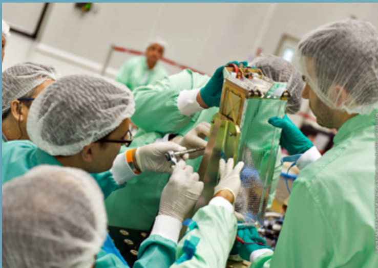
Fit checks for the CubeSats' P-POD on ASAP-S.
