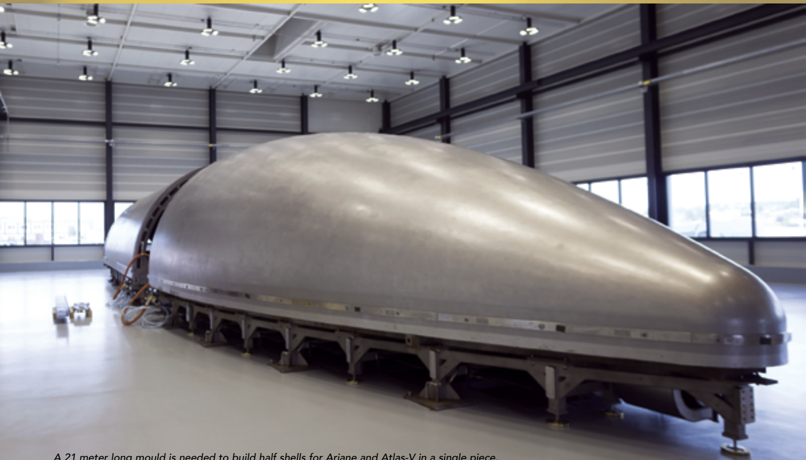
A 21 meter long mould is needed to build half shells for Ariane and Atlas-V in a single piece. Photo is courtesy of RUAG Space.
