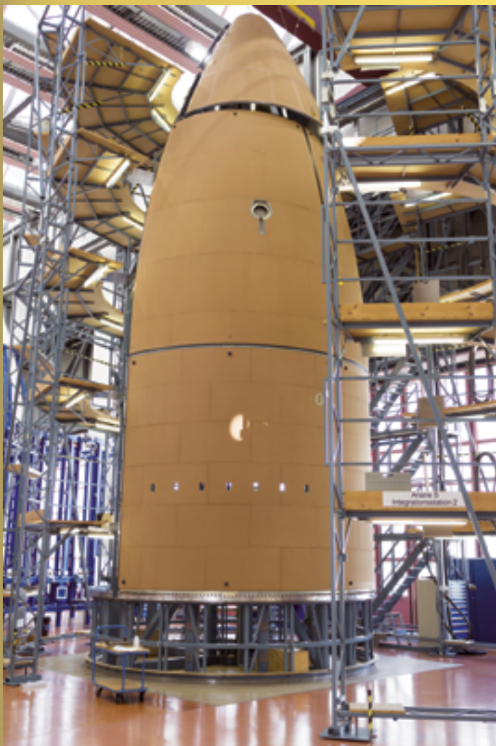
Today an Ariane Fairings is assembled into two half shells of seven elements each, in a meticulous manual process. Photo is courtesy of RUAG Space.
