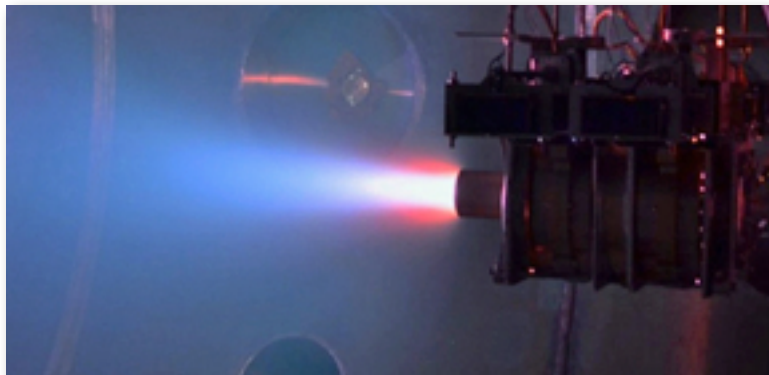
Elwing's E-IMPACT thruster firing at NASA MSFC's Propulsion Research and Development Laboratory.
