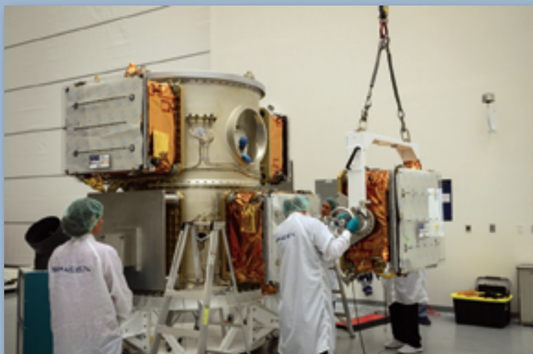
ORBCOMM's launch team installing the OG2 satellites on Moog's ESPA ring dispenser. Photo courtesy of SpaceX.
