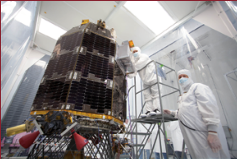
Engineers at NASA's Ames Research Center, Moffett Field, California, prepare NASA's Lunar Atmosphere and Dust Environment Explorer (LADEE) Observatory for acoustic environmental testing. Image credit: NASA Ames
