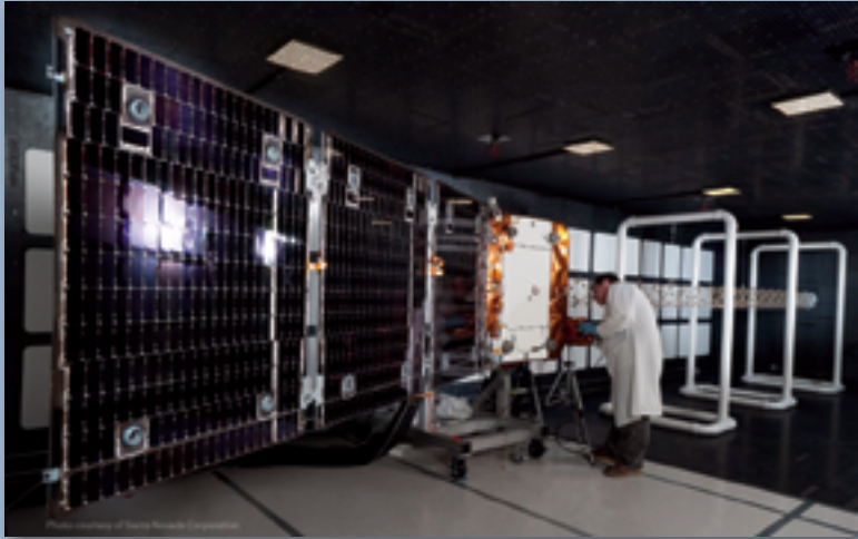
An ORBCOMM technician prepares OG2 satellite for electromagnetic compatibility testing. Photo courtesy of Sierra Nevada Corporation.
