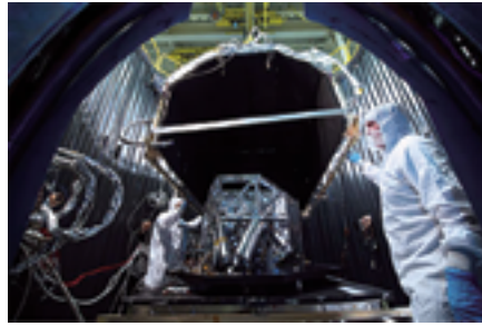
NASA testing the Webb Telescope's MIRI thermal shield. Image Credit: NASA/Chris Gunn.
