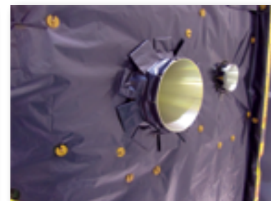
Details of the Aldo Paraboni (TDP 5) Payload Q-band and Ka-band horns, after final insulation installation in Kourou. Photo is courtesy of Airbus Defence and Space.
