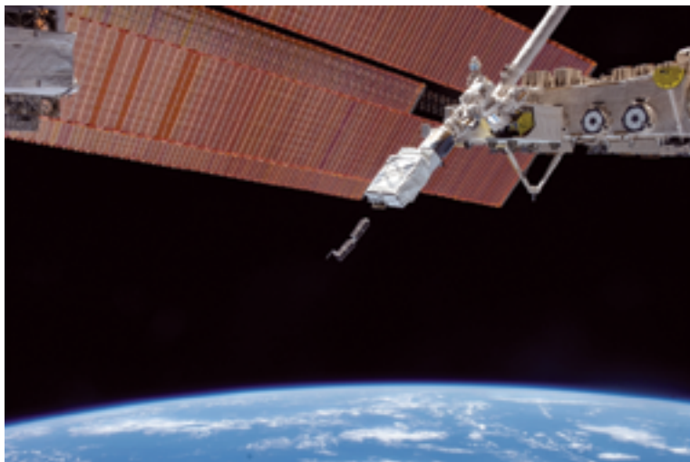
The Small Satellite Orbital Deployer (SSOD), in the grasp of the Kibo laboratory robotic arm, is photographed by an Expedition 38 crew member on the International Space Station as it deploys a set of NanoRacks CubeSats.
