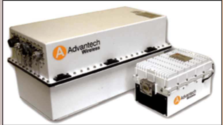
Figure 1. (Left) 50W Ku-band GaAs based SSPA (2006 generation), versus (Right) 50W Ku-band GaN SSPA (2010 generation)
