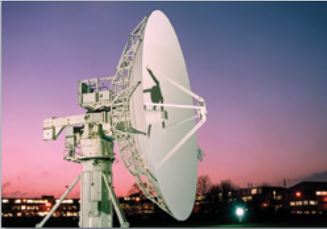
RAL Space is the primary operator for UKube and has established a UHF/VHF ground station, which commands the satellite. A 2.4m S-band antenna will be used to provide data downlink for UKube. These two systems will be able to support amateur satellites within the international community.
