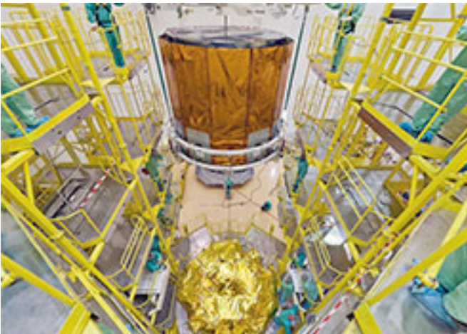
Gaia being lowered onto the Fregat stage. Photo courtesy of ESA.
