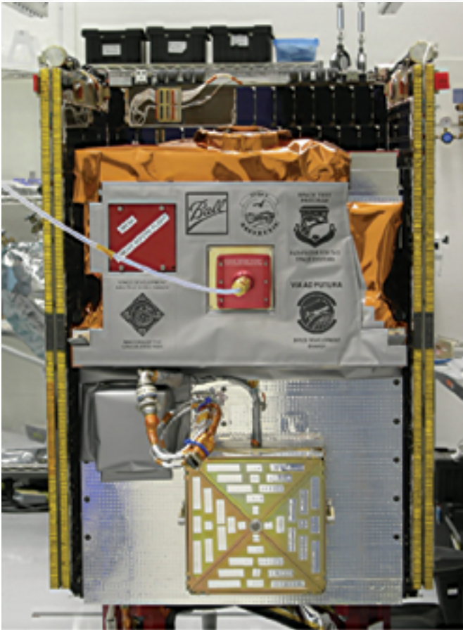
Ball's STP-SIV series of satellites is built on the Ball Configurable Platform (BCP) 100. Photo courtesy of Ball Aerospace.
