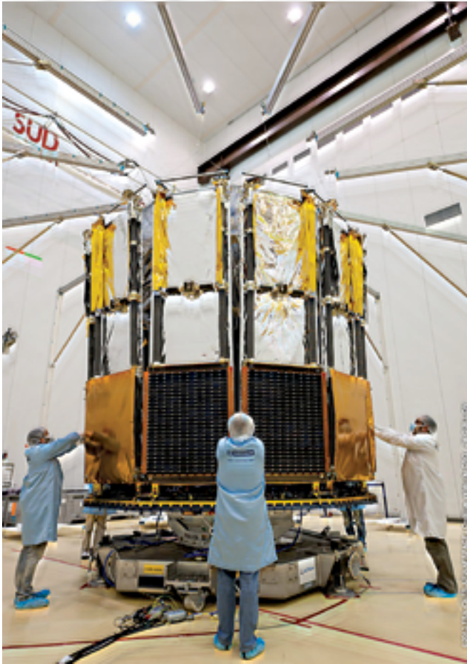
Engineers from SENER and Astrium stow Gaia's Deployable Sunshield Assembly (DSA) against the spacecraft, in the S1B cleanroom at the Centre Spatial Guyanais in Kourou, French Guiana. This photo is courtesy of ESA-CNES-Arianespace Optique Vidéo du CSG—JM Guillon
