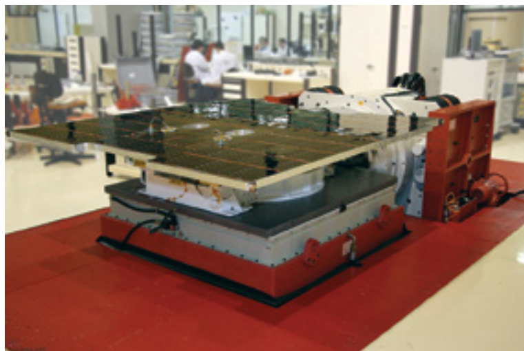
Satellite undergoing a shaking test.
