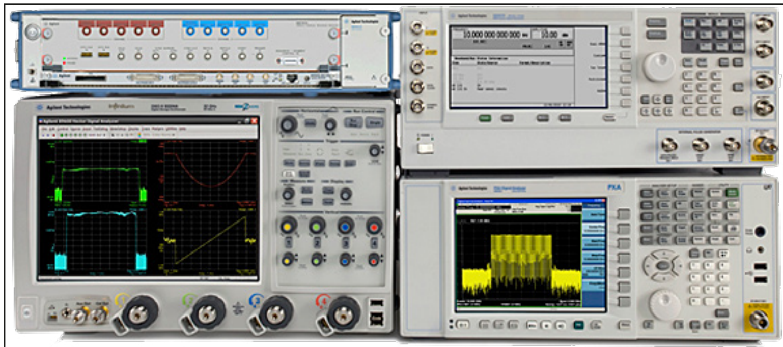
Figure 1: This four-instrument test setup enables testing of both receivers and transmitters.
