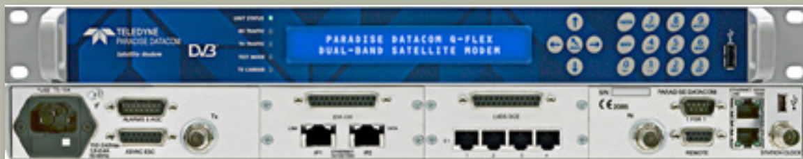
The front and back panels of the Q-Flex Modem.
