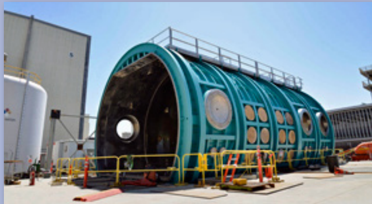
SSL's new Thermal Vacuum Chamber, under construction. Photo courtesy of SSL.
