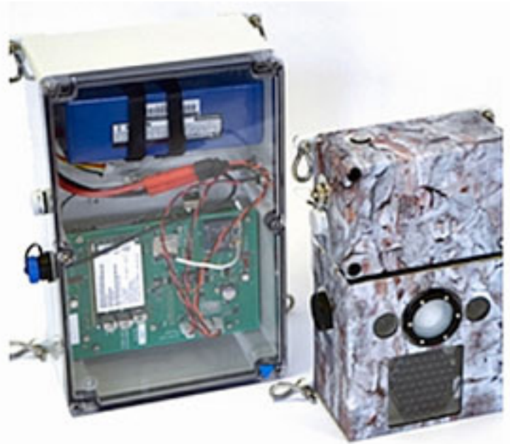
The satellite connected, motion triggered, camera, part of the Instant Wild project.
