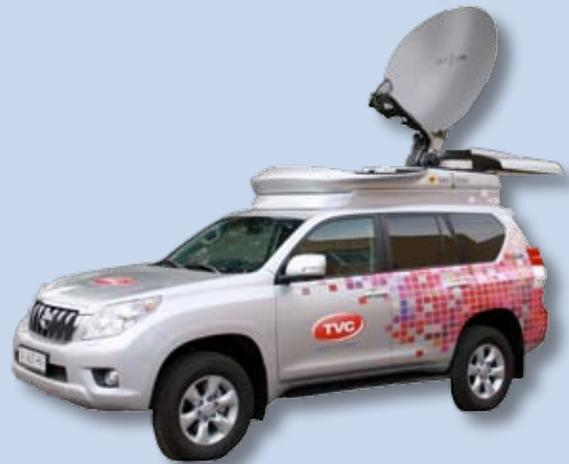
**Cover Image:** Built into a Toyota Land Cruiser by Lithuanian systems integrator TVC, KTK's DSNG station features a SWE-DISH/Rockwell Collins Drive Away Antenna system, two Ericsson Voyager II multi-format integrated DSNG encoders, and two fully redundant Ericsson RX8200 advanced modular receivers. This fully operational HD live production system connects with TV studios and Outside Broadcast vehicles and is being used for live broadcasting. DSNG Vehicle Photo Credit: TVC
