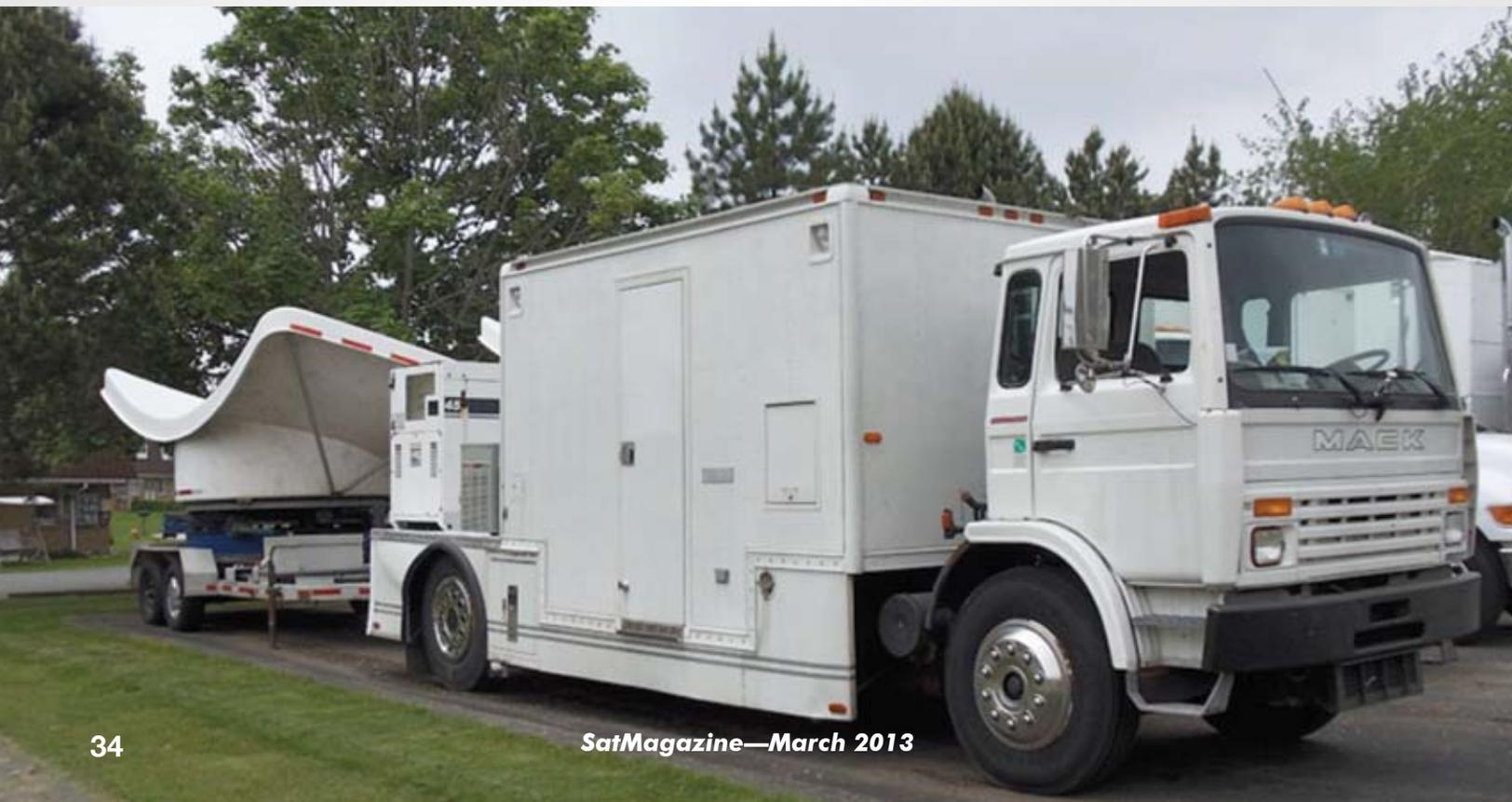
truck chassis, with a large box body. These trucks could be used to uplink to any satellite needed in order to transfer video and audio from any event that was newsworthy.
