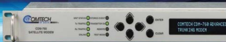
1 kbps – 150 Mbps • Up to 314 Mbps Simplex & 628 Mbps Duplex with 8PSK / 16APSK / 32APSK • > 1.2 Million PPS • 5%, 10% and 15% Rolloffs • Upgradeable to DVB-S2-EB1, DVB-Sx & DVB-S3
