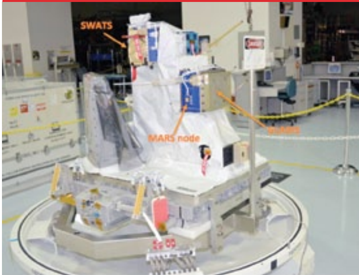
The STP-H4 complement is pictured here prior to encapsulation and shipment to Japan. NRL's three experiments—SWATS, MARS, and GLADIS—are identified. (Photo: DoD Space Test Program)
