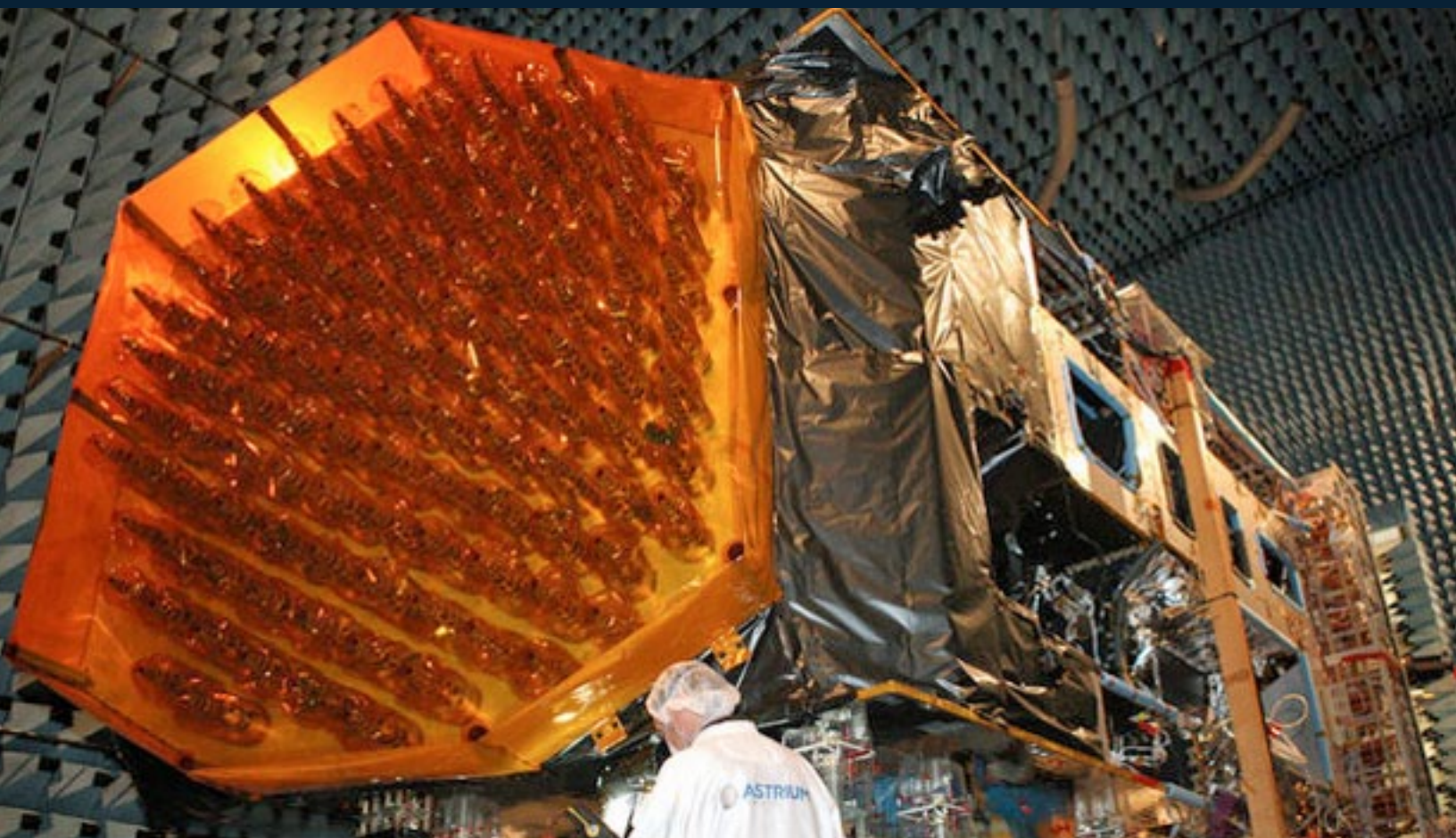
The Alphabus product line is Europe's response to market demand for increased broadcasting services. It accommodates missions with up to 22kW of payload power and mass up to 2 tons. As a high-power, multi-purpose platform, it gives European industry an unprecedented and unique position in the global telecom market. Photo courtesy of ESA.
