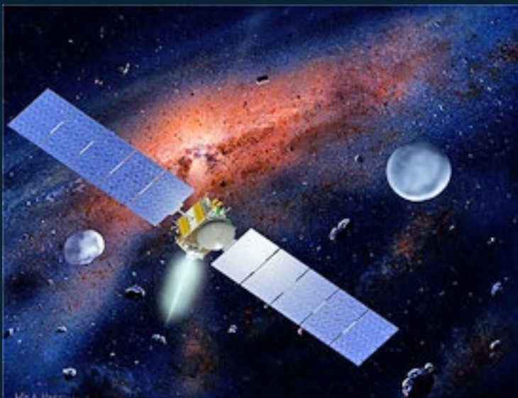
The Dawn satellite, powered by a xenon ion propulsion unit, image courtesy of NASA. The protoplanet approach phase for this spacecraft will use electricity to ionize and accelerate xenon for thrust generation
