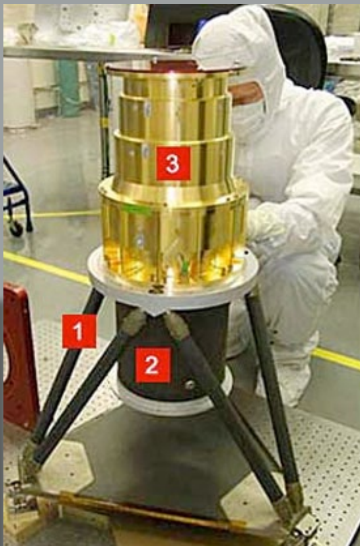
The GOES-R GLM instrument. 1=Sensor Unit Mechanical Support Structure. 2=Metering Tube. 3=Optical Assembly. Photo is courtesy of NOAA/NASA.
