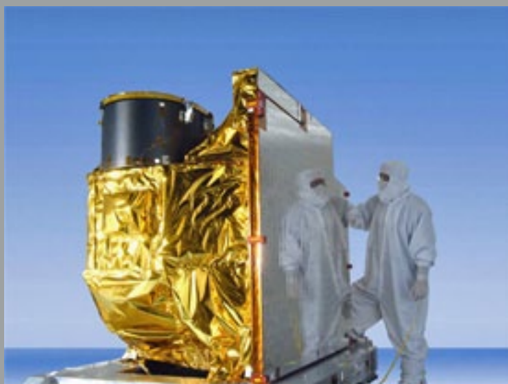
A cornerstone of the mission is the 16-channel ABI instrument, shown above. Photo courtesy of NOAA/NASA.
