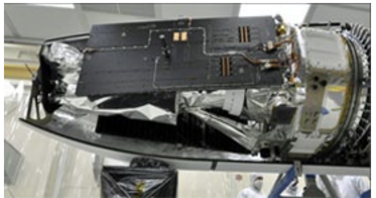
The IRIS spacecraft will use an ultraviolet telescope to look at a small area of the sun to answer detailed questions. Photo courtesy of NASA.
