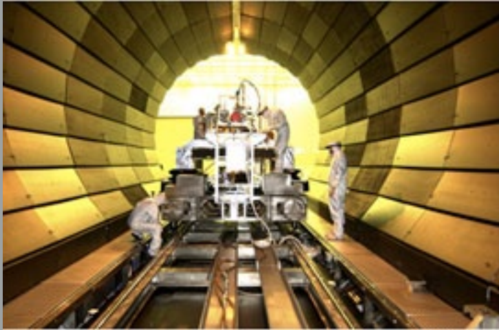
Solar X-Ray Imager Testing in the X-Ray Calibration Facility (XRCF). Photo Courtesy of NASA's Marshall Space Flight Center.
