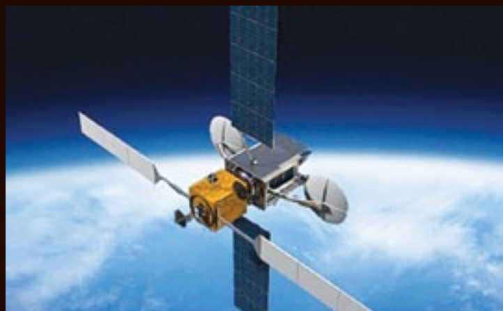
The ViviSat MEV is designed to attach to an existing satellite that is in dire straits as its propellant is dangerously low—the MEV would take over station keeping and attitude control of the target satellite while accomplishing its mission.
