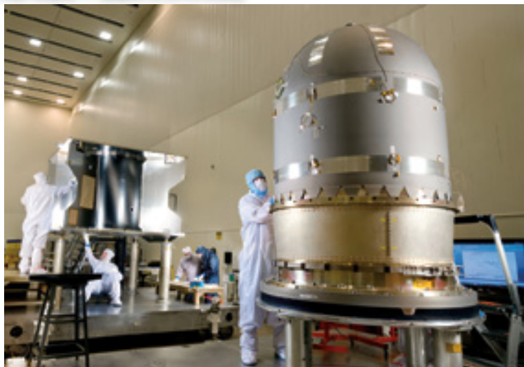
This photo shows the large hydrazine propellant tank prior to integration with the core structure of the MAVEN spacecraft at a Lockheed Martin clean room near Denver. The tank will hold 450 gallons of hydrazine propellant and is 6 feet 2 inches tall. The tank was built by ATK Aerospace Group, Commerce, California. The primary structure in the background is cube shaped at 7.5 feet x 7.5 feet x 6.5 feet high. Built out of composite panels comprised of aluminum honeycomb sandwiched between graphite composite face sheets, the entire structure only weighs 275 pounds. Photo is courtesy of Lockheed Martin.
