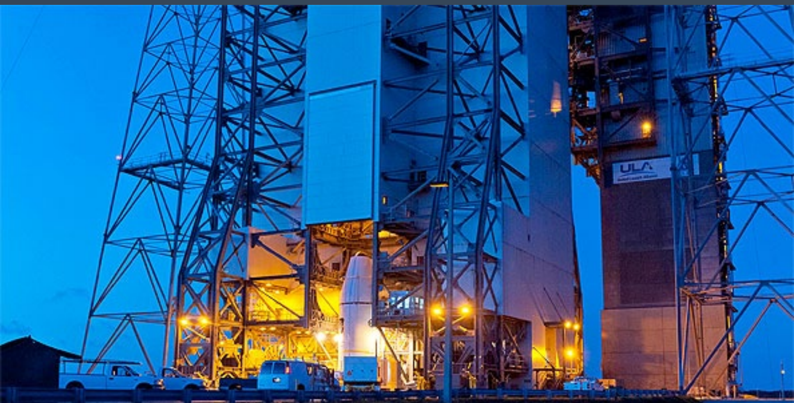
The U.S. Air Force's GPS IIF-3 satellite, encapsulated inside its 4-meter diameter payload fairing, is mated to a United Launch Alliance Delta IV launch vehicle. Photo ULA.
