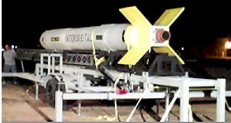
Photo of a Common Propulsion Module Test Vehicle (CPM TV) on its Mobile Launch Trailer (MTA), photo courtesy of IOS.
