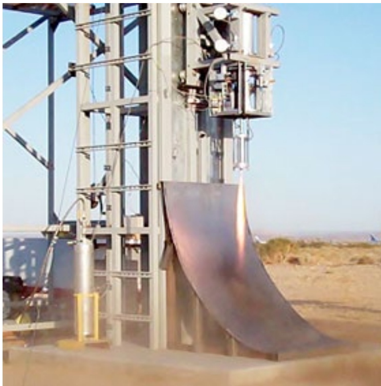
Successful test firing of the IOS CPM vernier rocket engine
