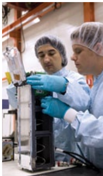
University of Bucharest's Goliat being integrated into the first P-POD. Credits: ESA / A. Reyes
