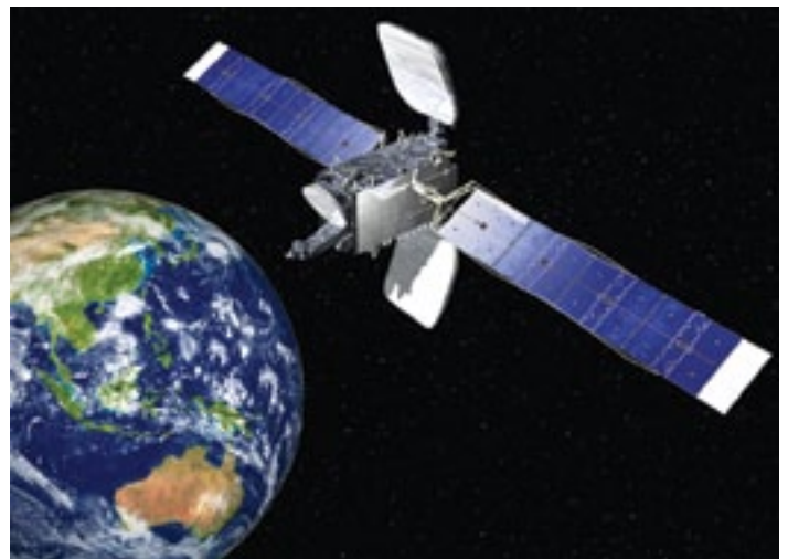
The SES-8 satellite, expected to launch in 2013, will be slotted at 95 degrees East and will carry 33 high power Ku-band transponders and will be co-positioned with SES-6. Image is courtesy of Orbital Sciences Corporation.
