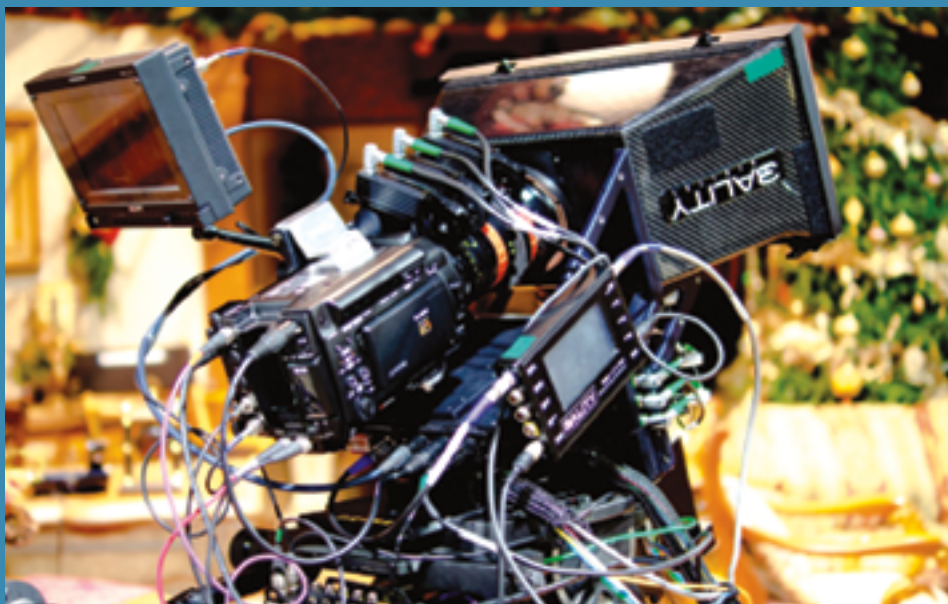
Sony's PMW-F3's on a 3ality TS5 rig, as used on the experimental shoots
