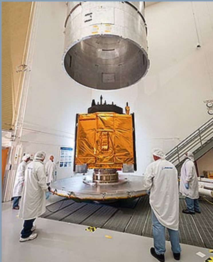
Boeing technicians prepare a GPS satellite for mass properties testing at the company's facility in El Segundo. Mass properties testing ensures that a satellite meets weight, center of gravity, dynamic balance, and moment of inertia requirements in preparation for launch and operation. Boeing GPS testing uses a robust spin rate of 40 rpm. Two GPS IIF satellites are currently in service, two are complete and await launch, and eight are in various stages of manufacture. Photo courtesy of Boeing.
