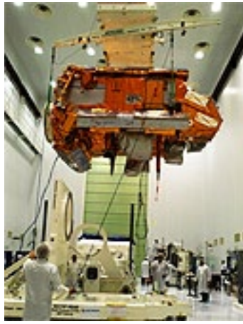
The MetOp-B satellite payload module being lowered onto the trolley for its first inspection after arrival at the launch facilities in Baikonur. Credit: ESA
