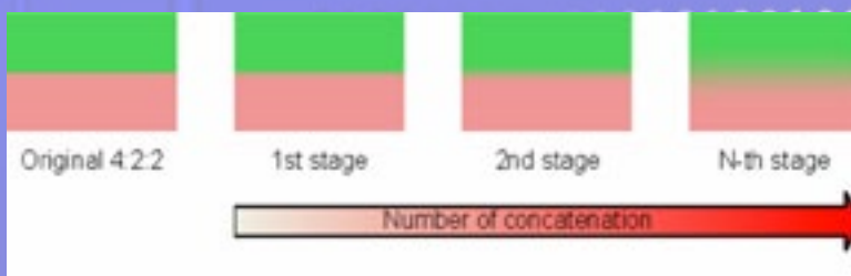
Figure 1. Degradation of a 4:2:0 chroma component in concatenated operations
