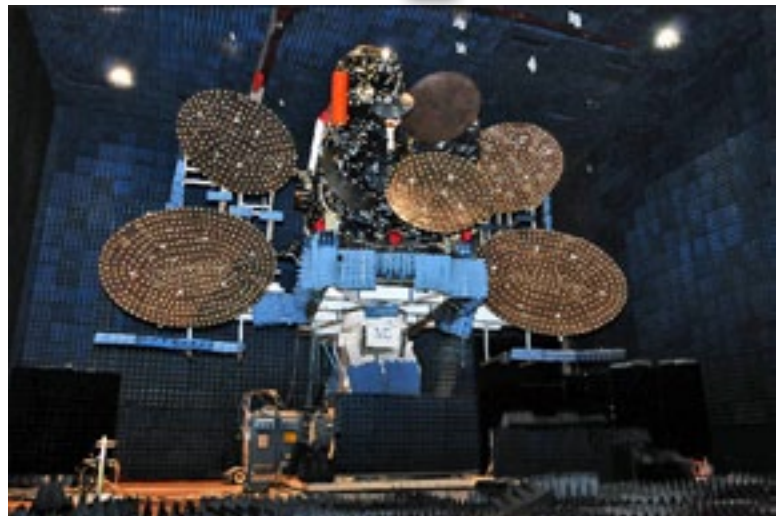
NSS-12 deployed in compact antenna test range. Photo courtesy of Space Systems/Loral.
