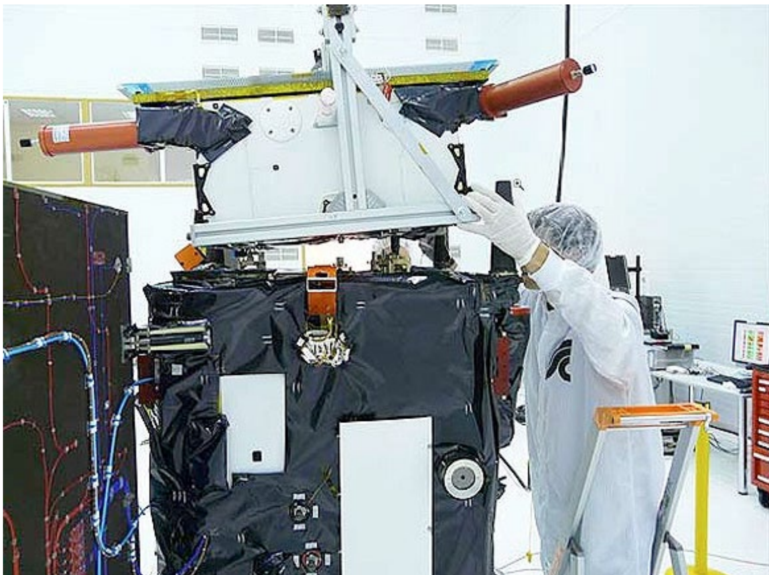
Tango (top) and Mango (bottom) are mated into their launch configuration in May of this year. Photo is courtesy of SSC.
