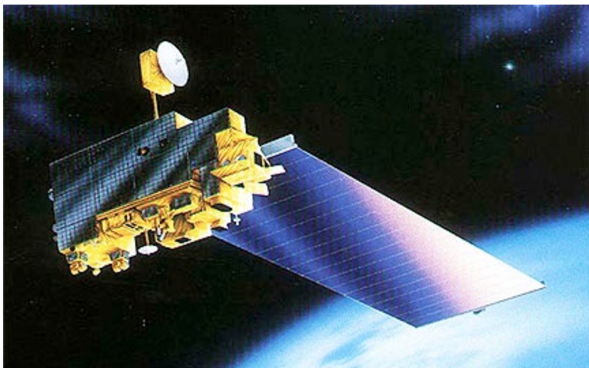
The Advanced Spaceborne Thermal Emission and Reflection Radiometer is an imaging instrument that is flying on NASA's Terra satellite as part of the space agency's Earth Observing System.
