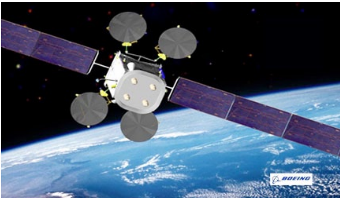
The Intelsat-22 satellite (IS-22) is one of four 702MP satellites ordered from Boeing by Intelsat Ltd. and will carry a UHF payload that will provide service to the Australian Defence Force. The launch of this satellite is scheduled for 2012. Image courtesy of Boeing.
