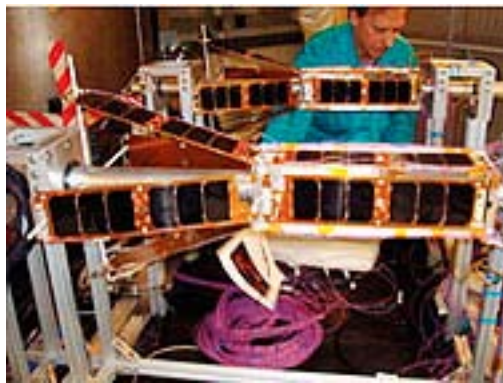
Two QbX CubeSats being prepared for TVAC testing at NRL's Spacecraft Checkout Facility. Credit: U.S. Naval Research Laboratory
