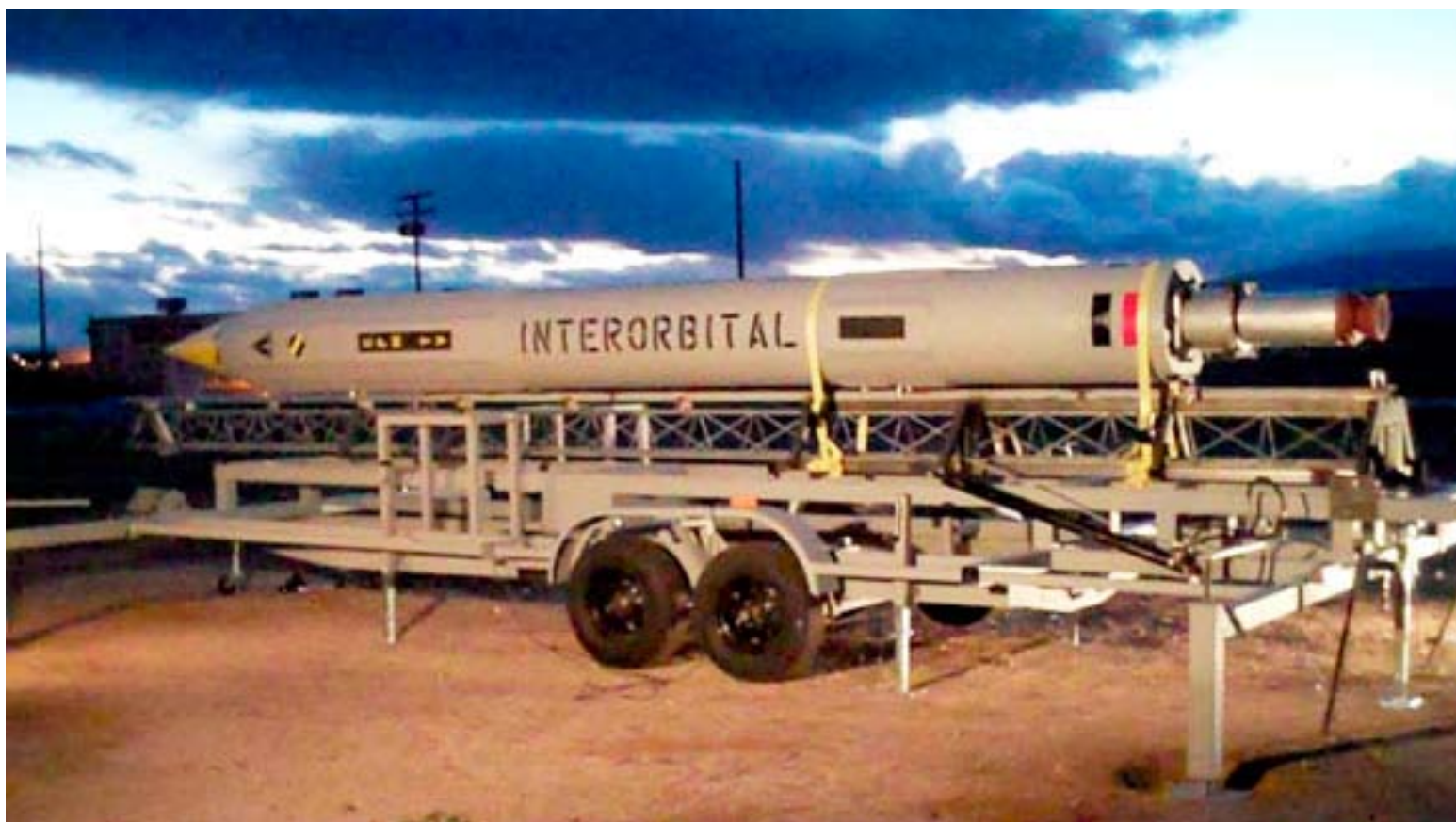
IOS CPM TV (Common Propulsion Module Test Vehicle) during Mobile Launch System lift test
