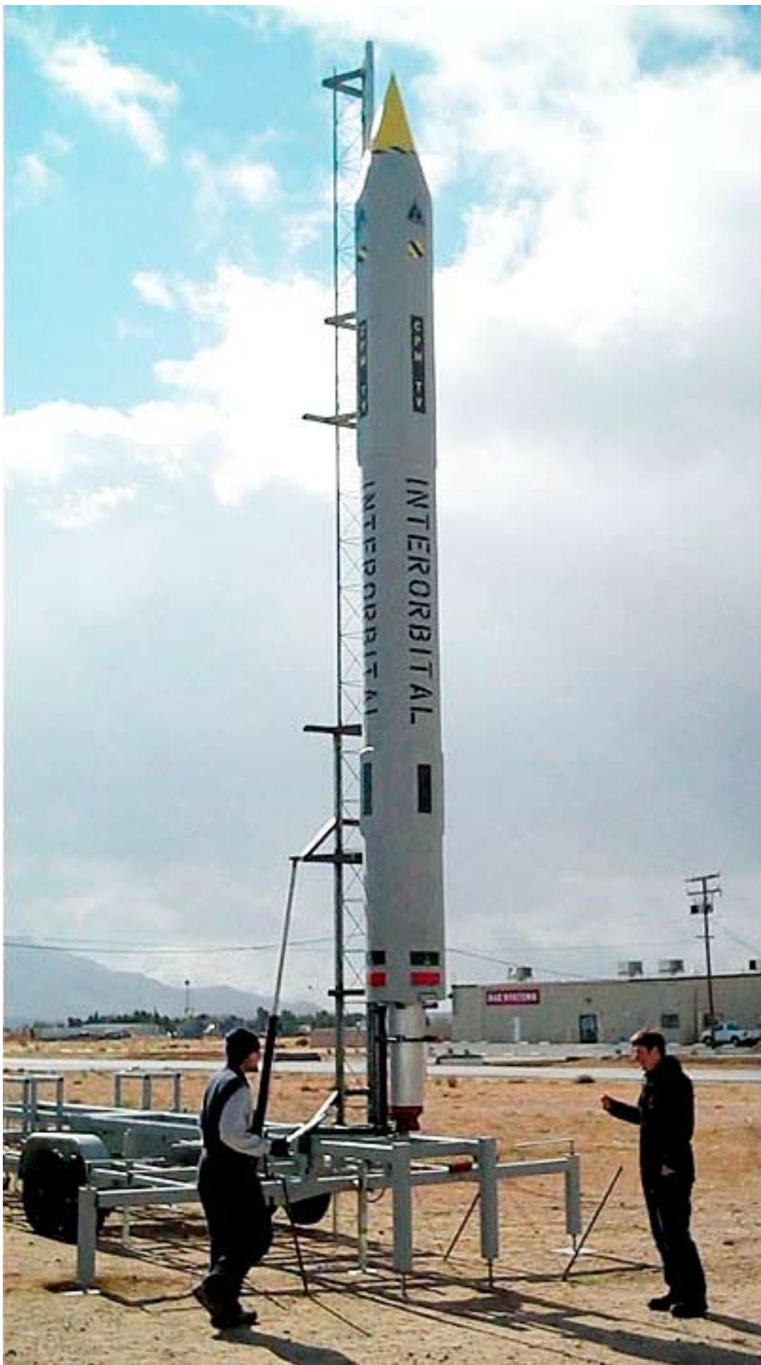
Spacecraft Technician Ryan Edblad and IOS President/CTO Roderick Milliron inspect the Common Propulsion Module during mobile launch system lift test at Mojave Spaceport
