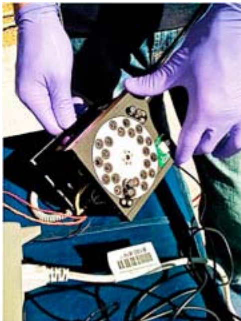
The O/OREOS chemistry cube contains 24 sample compartments and a spectrometer, all packed into a 10-cm 3 box.
