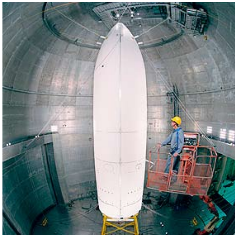
Preparation of a fairing for a separation test. Photo: NASA / GRC
