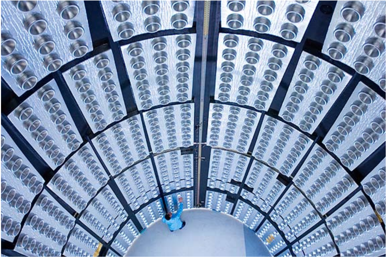
Acoustic absorbers inside a payload fairing. Photo: RUAG Space
