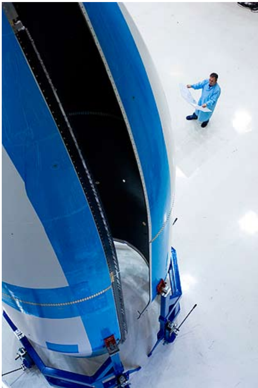
Payload Fairing for Vega. The new small European launcher is to have its maiden flight in 2011. Photo: RUAG Space
