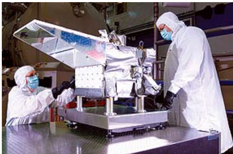
Raytheon technicians work on the Glory satellite's Aerosol Polarimetry Sensor (APS). The APS will explore the global distribution of aerosols and measure their effect on atmosphere. Glory will also carry the Total Irradiance Monitor, which will take measurements to help determine the Sun's direct and indirect effect on Earth's climate. Credit: Raytheon
