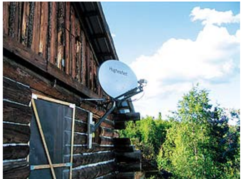
Satellite internet connections, like this HughesNet setup in Alaska, allow people in remote areas to access the internet at broadband speeds. Credit: John Bollinger
