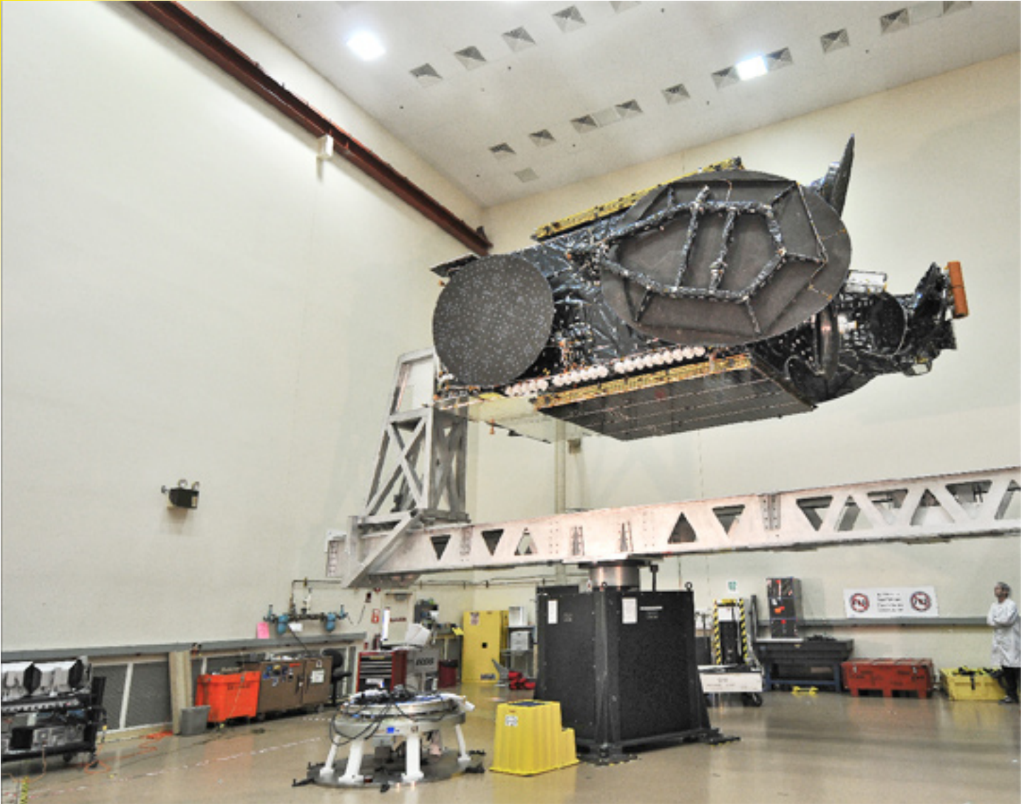
NSS-12 undergoing gravity spin test at SS/L—image courtesy of SS/L
