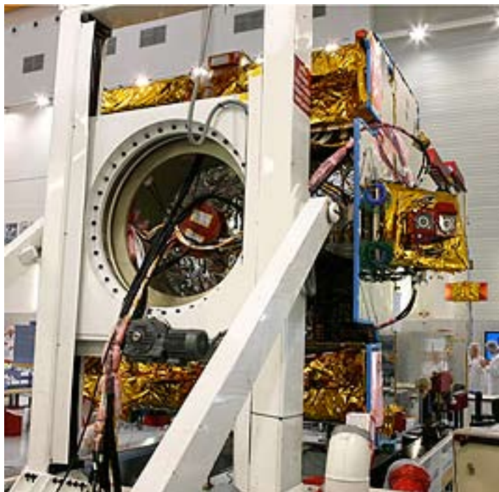
Eutelsat's Ka-Sat chemical thruster, which can be seen behind the ring that's been bolted onto the white trolley.
