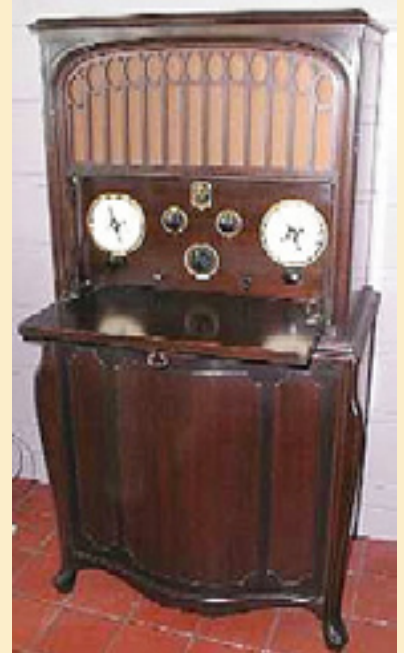
Circa 1924 — The RCA-GE Radiola Super-VIII, a six tube, catacomb-type, superheterodyne chassis with built-in antenna and built-in horn speaker.
