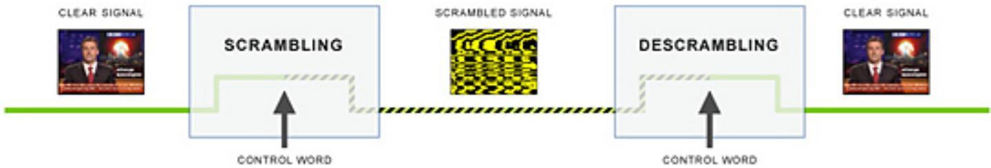
**Figure 1 — The clear signal is fed into the scrambler which encrypts using the Control Word. The descrambler uses the same Control Word to recreate the original clear signal.**
