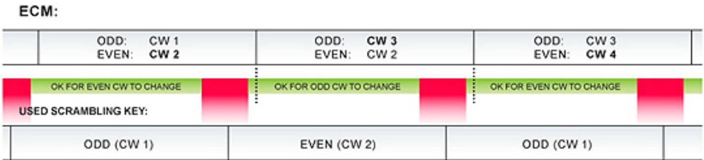
**Figure 3 — The change of the ECM has to happen a certain time after the Control Word used to scramble the signal has changed. Similarly the change of the ECM has to happen some time before this new Control Word will start to be used to scramble the signal.**
