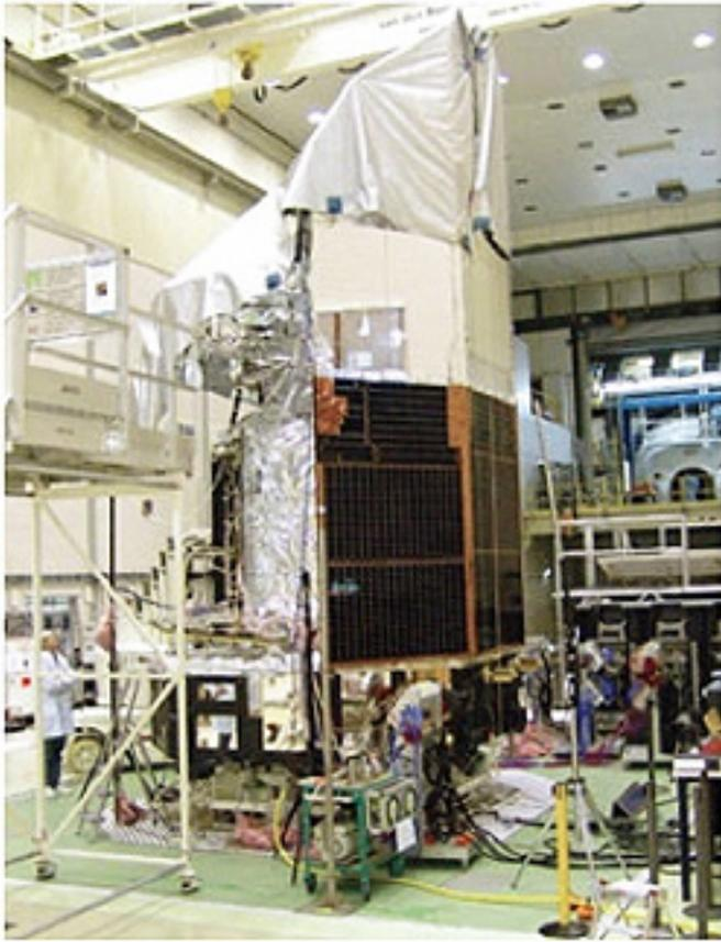
*HERSCHEL being prepared to undergo vibration testing. Herschel will be the largest space telescope of its kind when launched. Herschel's 3.5 m diameter mirror will collect long-wavelength, infrared radiation from some of the coolest and most distant objects in the Universe.*
