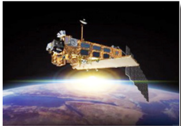
Envisat satellite, whose payload carries nine Earth observation instruments
