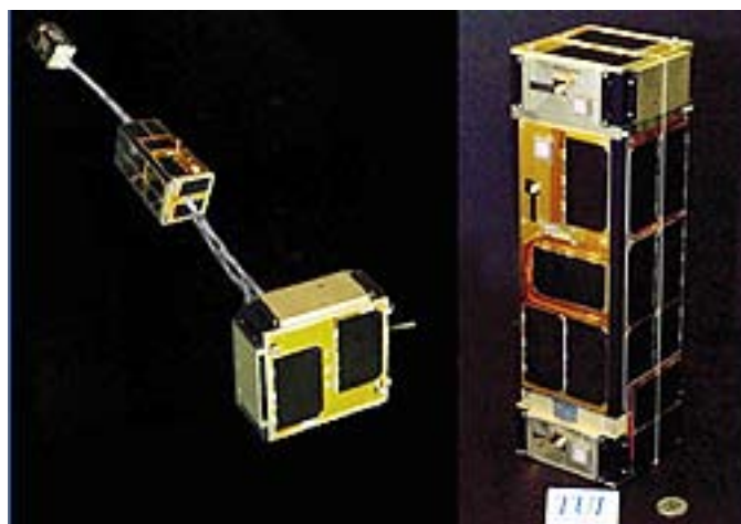
MAST—deployed (l.) and launch configuration (r.)
