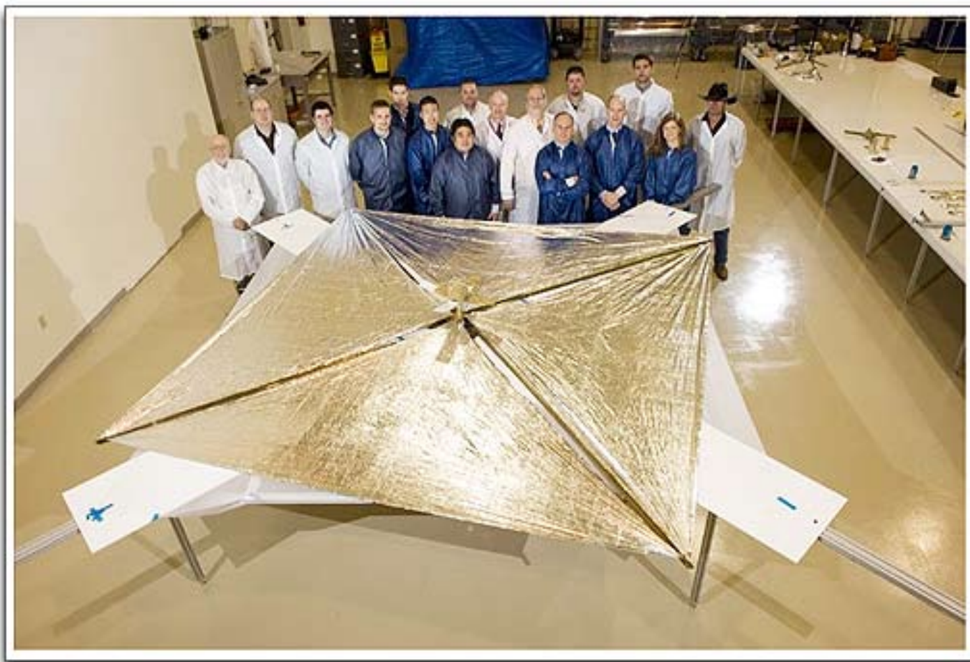
NanoSail-D poses after a successful laboratory deployment test. Edward E. Montgomery's team from the Marshall Space Flight Center worked in cooperation with Elwood Agasid's Ames team on deploying the NanoSail-D solar sail.
