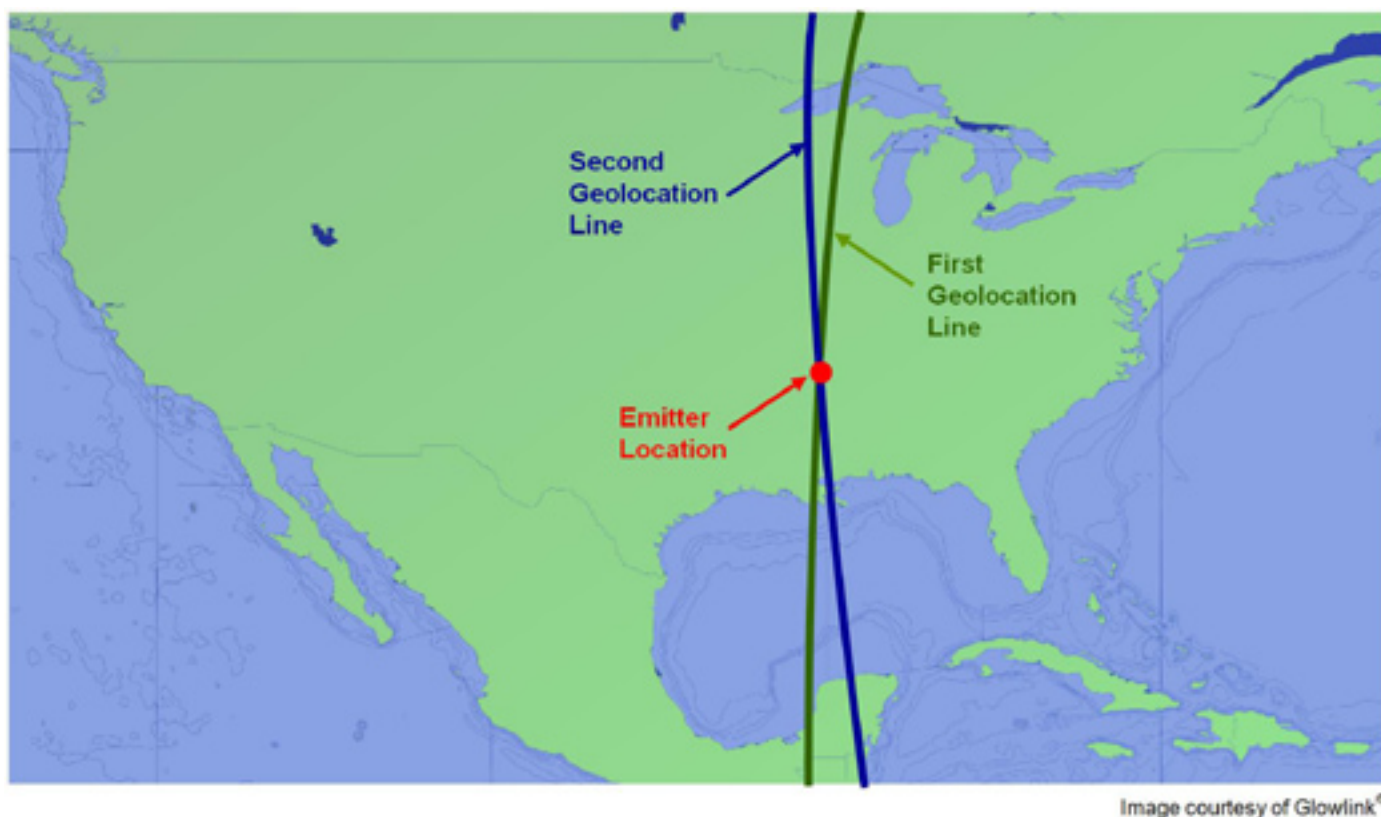
Figure 5 — Geolocating The Transmit Emitter Location
