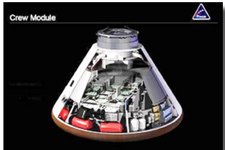
Cutaway image of Orion crew module, courtesy of NASA
