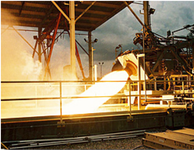
Demo of Deep Throttle Engine Capability, courtesy TGV Rockets
