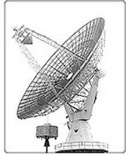
Huge 85-foot antenna at Point Mugu, Calif., relayed TV signals from Syncom 3, shown full size at bottom left.
