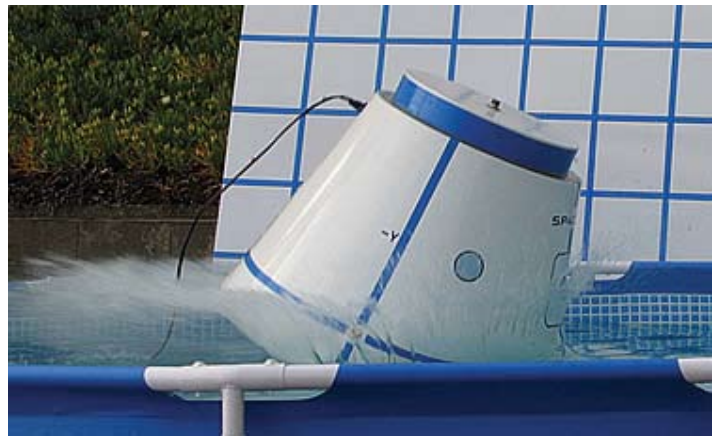
One-third scale Dragon capsule model drops into testing pool Photo courtesy: Space X
