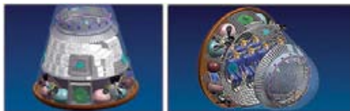
Left: Dragon with pressurized section filled with cargo Right: Dragon with pressurized section fitted with seats, people, and life support
